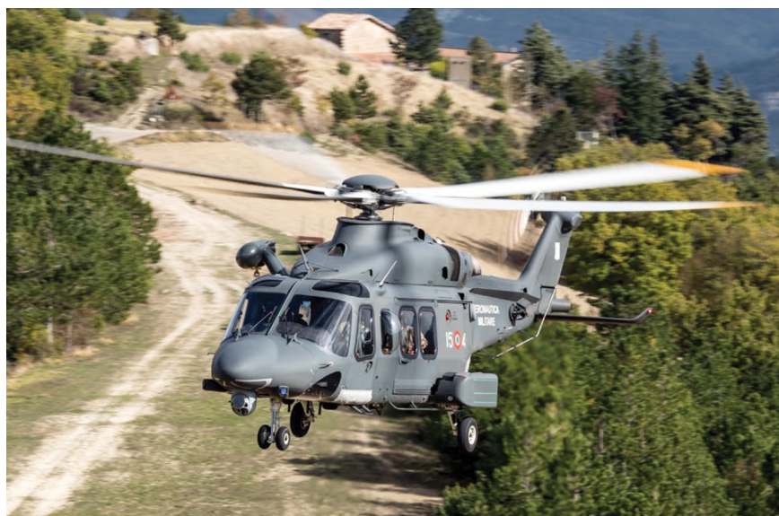
This HH-139A shows the FLIR and hoist to enable SAR duties
