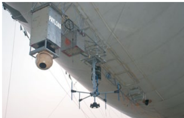
EO and COMINT payloads mounted on Aerostat.
