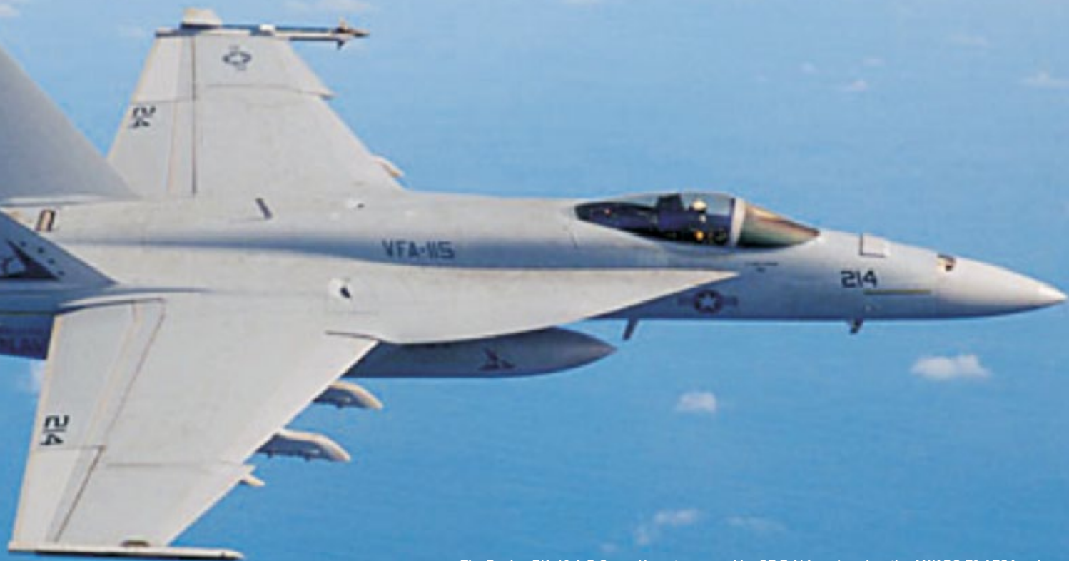
The Boeing F/A-18 A-D Super Hornet, powered by GE F 414 engines has the AN/APG-79 AESA radar. Other advantages include carrier capability and a very wide range of integrated weapons.
