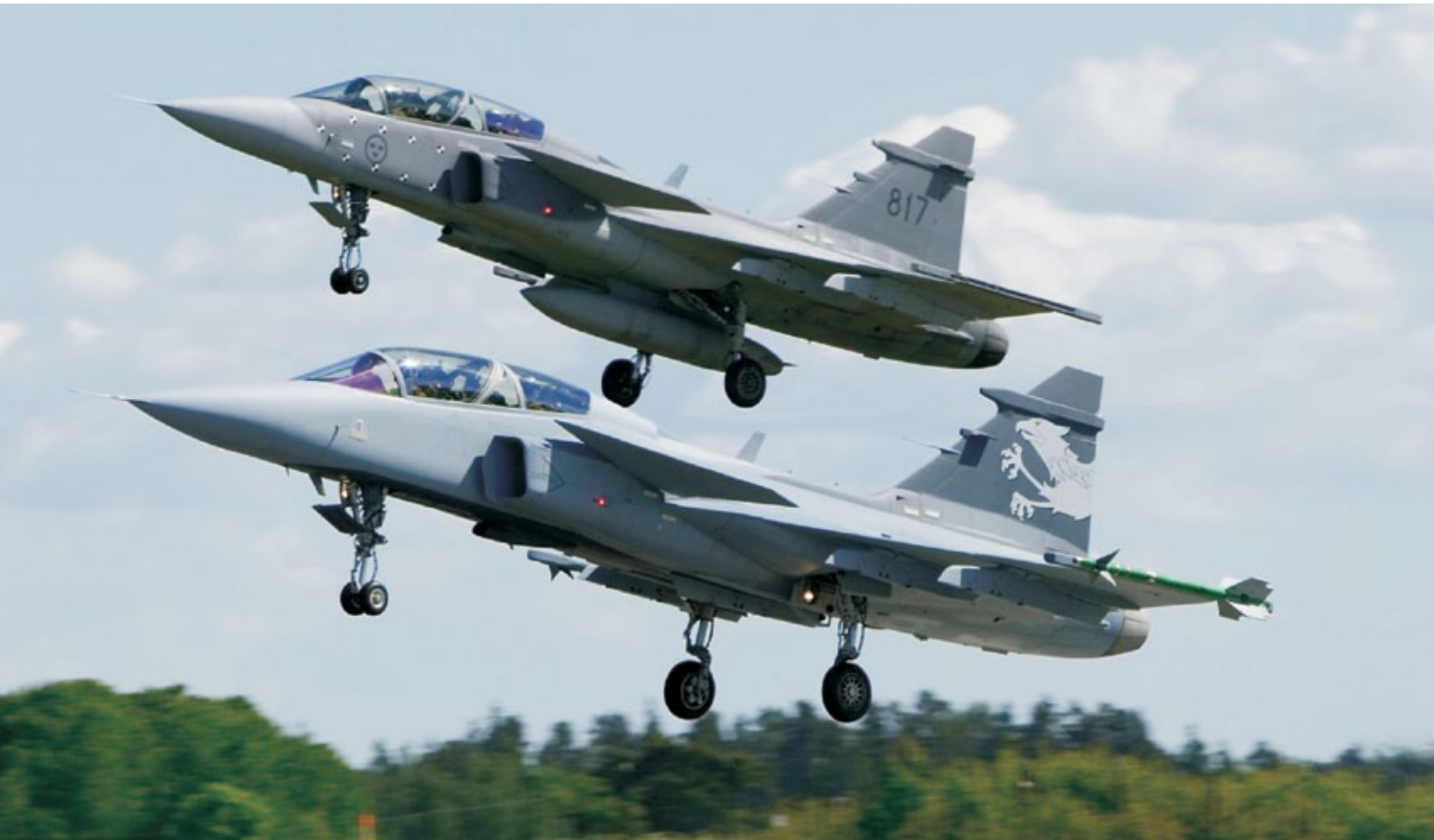
The Saab Gripen IN next generation multi-role combat aircraft has evolved from the Gripen C, is powered by a GE F414 turbofan engine and described as "a true 4+ generation lightweight fighter and significantly more capable than category competitors".
