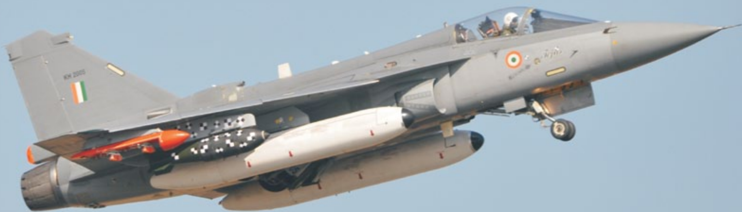
PV-3 (KH-2005), the first production variant takes off with underwing stores including drop tanks and free fall bombs.
