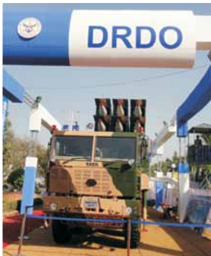
DRDO displayed the Prahar tactical ballistic missile (TBM) in 3x2 configuration mounted on a Tata transporter.
