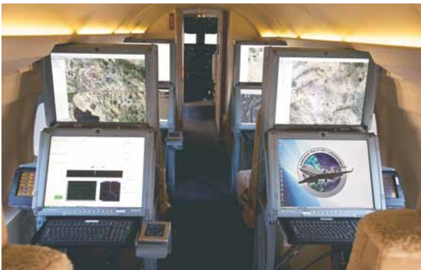
The interior can be configured for up to 8 operator stations, depending on the role required (LM photo)
