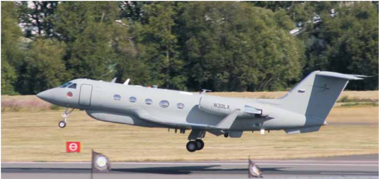
The Dragon platform aircraft demonstrator takes off showing its large canoe shaped SAR radar housing below the fuselage. (LM photo)
