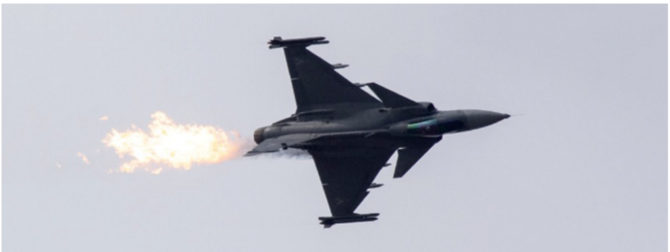
This Hungarian JAS.39C Gripen flew a stunning display, with the spectacular fuel 'dump and burn' as highlight. Seemingly on fire, this technique is used to dump fuel in an emergency situation, where a quick landing is needed but the aircraft is still too heavy to safely land
