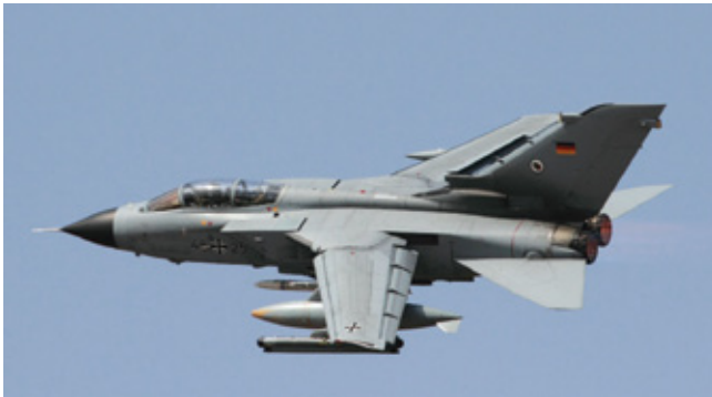
The German Luftwaffe recently announced it will order more Eurofighter EF2000 jets. Some of these will be of a still to develop ECR version, intended to replace the Tornado ECR fleet. In the meantime the venerable Tornado, designed by Germany, Italy and the United Kingdom in the seventies, is still going strong. Here it shows its topside with the swing wings in full forward position
