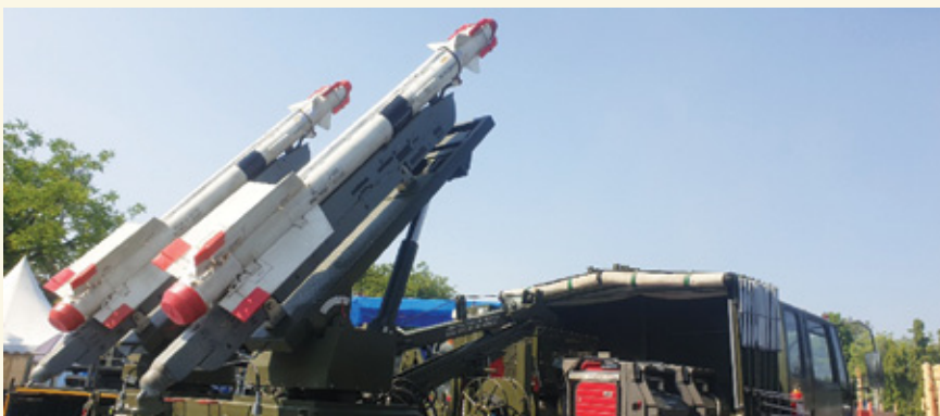
Samar air defence system with clever use of AAMs in the SAM role!
