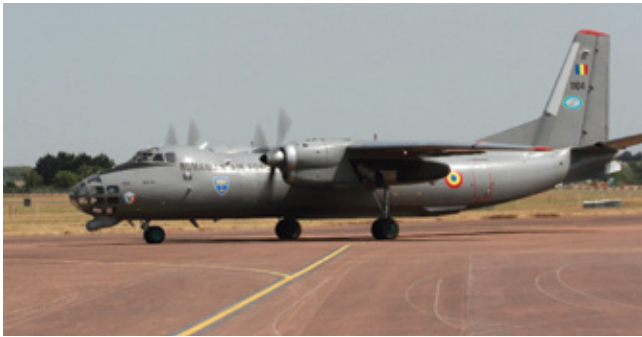
If the glass nose doesn't speak for itself enough, the badge on the nose of this Antonov An-30 saying "Patrula Aerofotogrammetrica" explains the role of this remarkable and rare aircraft. The Romanian Air Force still operates two of the almost 50 year old veterans, NATO reporting name 'Clank', for the Open Skies programme
