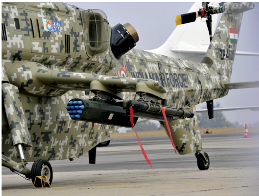
The Mistral ATAM air to air missile system for helicopters seen here on HAL's LCH.
