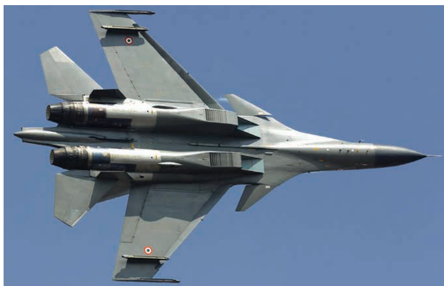
Large numbers of the Sukhoi Su-30MKI equip the Indian Air Force, this 'air dominance' fighter having long range capability and carrying several BVR air-to-air missiles including the Vympel NPO R-77 missile (export designation RVV-AE) missile seen above
