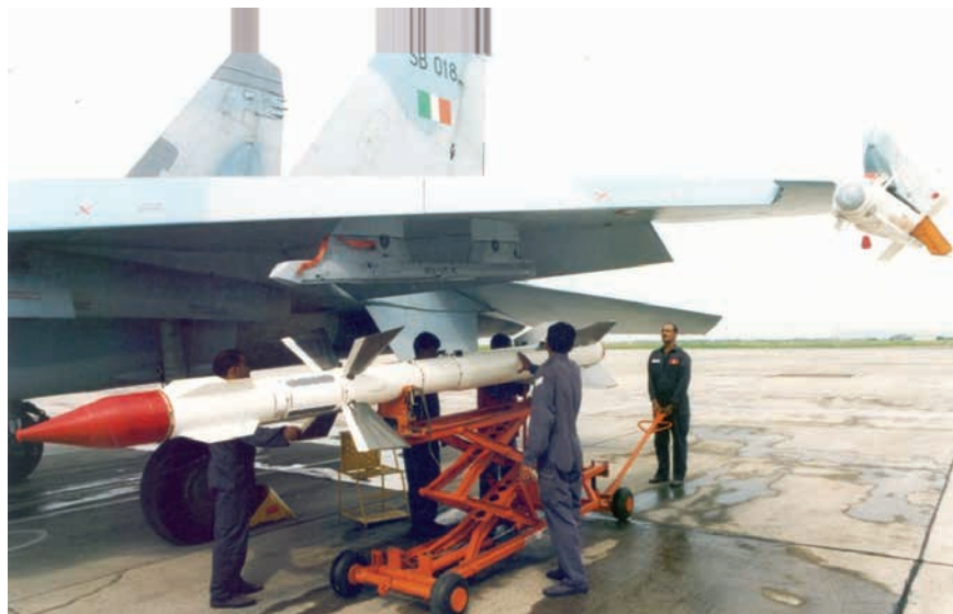
Large numbers of the Sukhoi Su-30MKI equip the Indian Air Force, this 'air dominance' fighter having long range capability and carrying several BVR air-to-air missiles including the Vympel NPO R-77 missile (export designation RVV-AE) missile seen above
