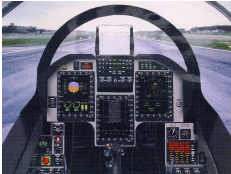
Smartly laid out: glass cockpit of the JF-17.
