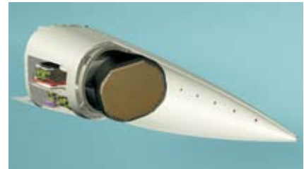
Selex Galileo Raven ES-05 AESA radar for the Gripen NG.
