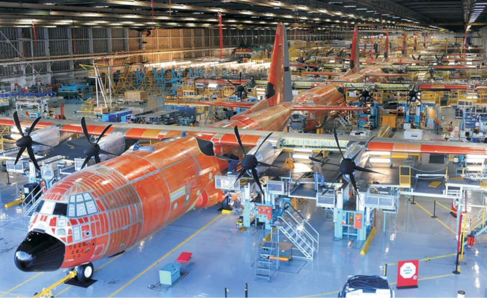
Nearly there! With engines installed, C-130Js in the final assembly line.
