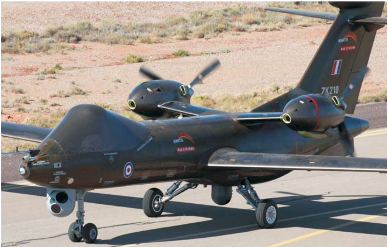
The BAE Systems Mantis is a new generation autonomous armed unmanned air system that may replace the current Predator/Reaper UAVs in service in Afghanistan.
