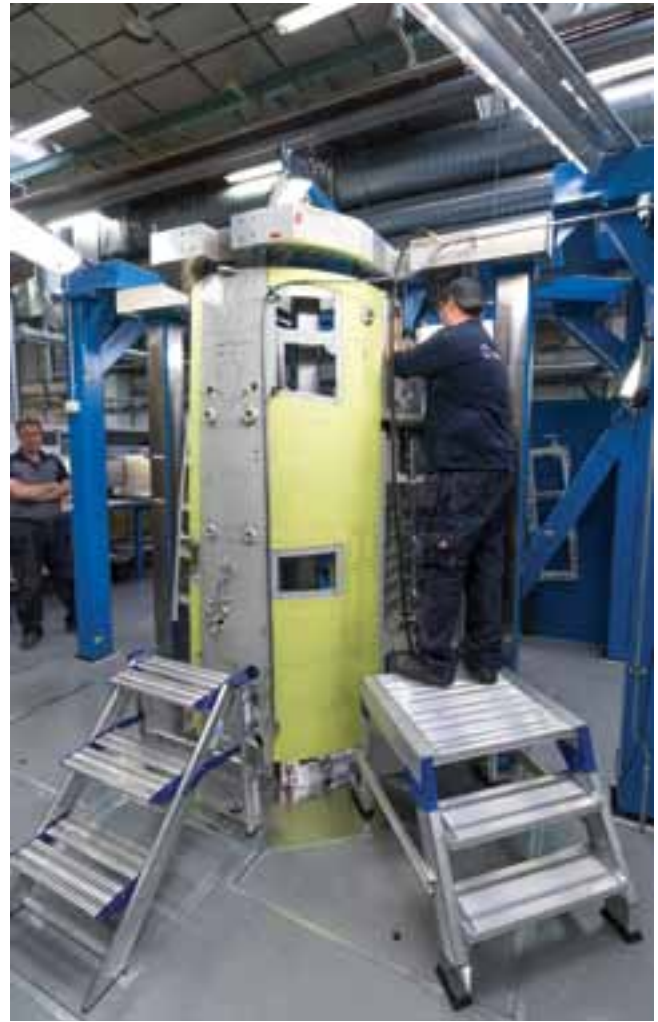
39-10 rear fuselage under assembly in a jig at Saab's Linköping facility
