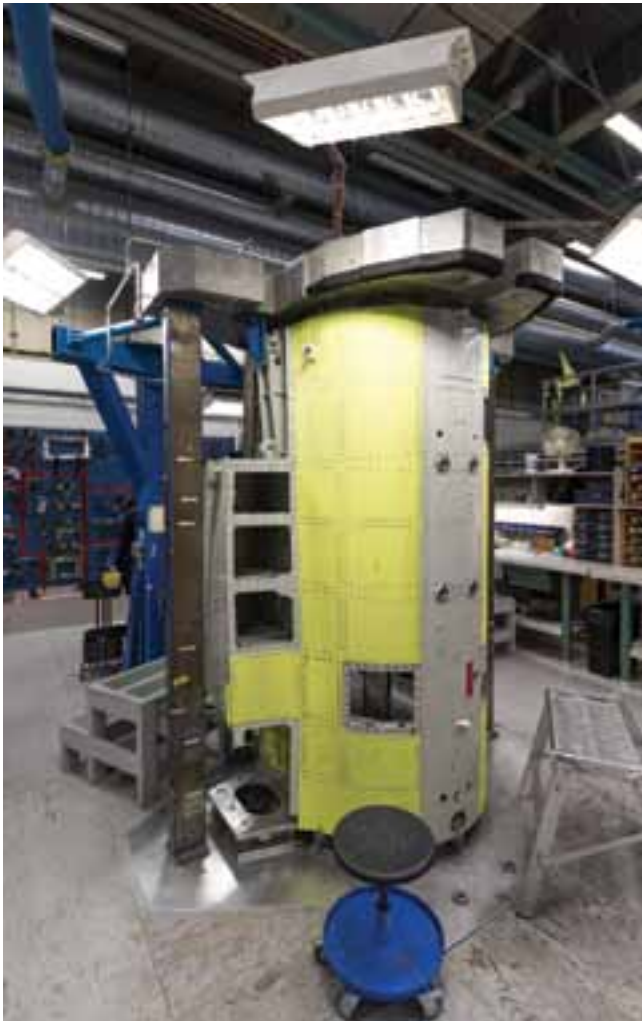
Gripen C/D rear fuselage being assembled in a jig – subtle differences are visible when compared to the Gripen E rear fuselage pictured to the right
