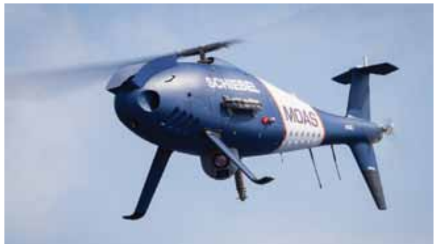
A Schiebel Camcopter S-100 with IAI Tamam POP 300 payload
