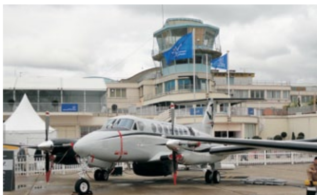
The Hawker Beechcraft King Air 350ER special mission aircraft on static display at Le Bourget. The aircraft is equipped with an under belly radar radome, a electro-optic/infrared (EO/IR) lift and fairing plus additional special mission equipment. It can be employed as an air ambulance or as a five-seat transport.
