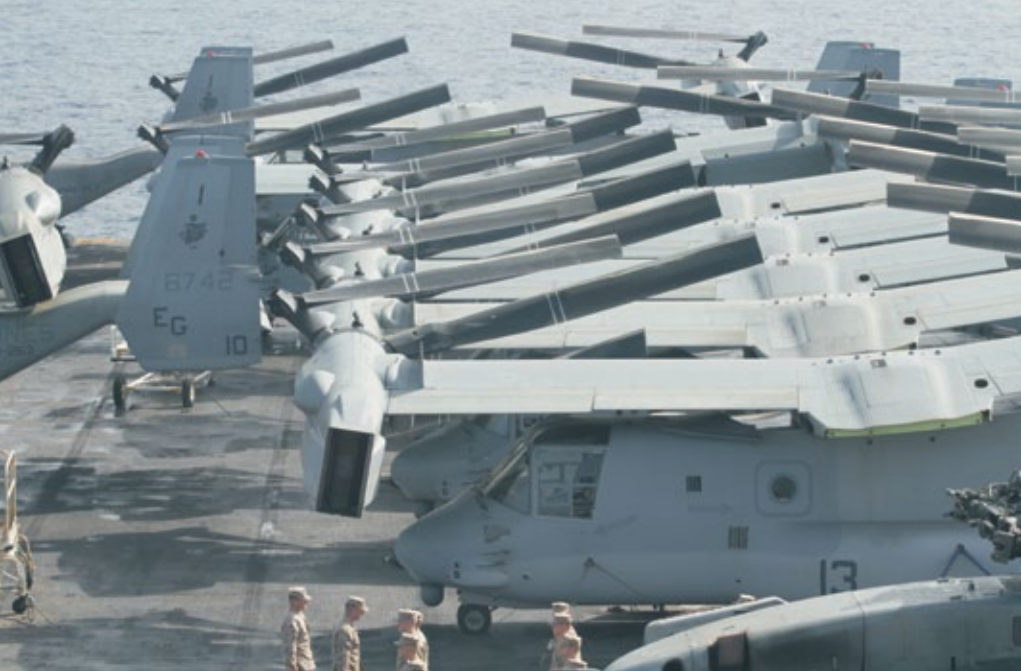
The MV-22 Osprey is capable of folding its wing and tilt the rotors in order to fit on the deck of a Landing Helicopter Deck. The maximum capacity onboard USS Bataan is limited to ten Ospreys mainly owed to the weight of these aircraft.
