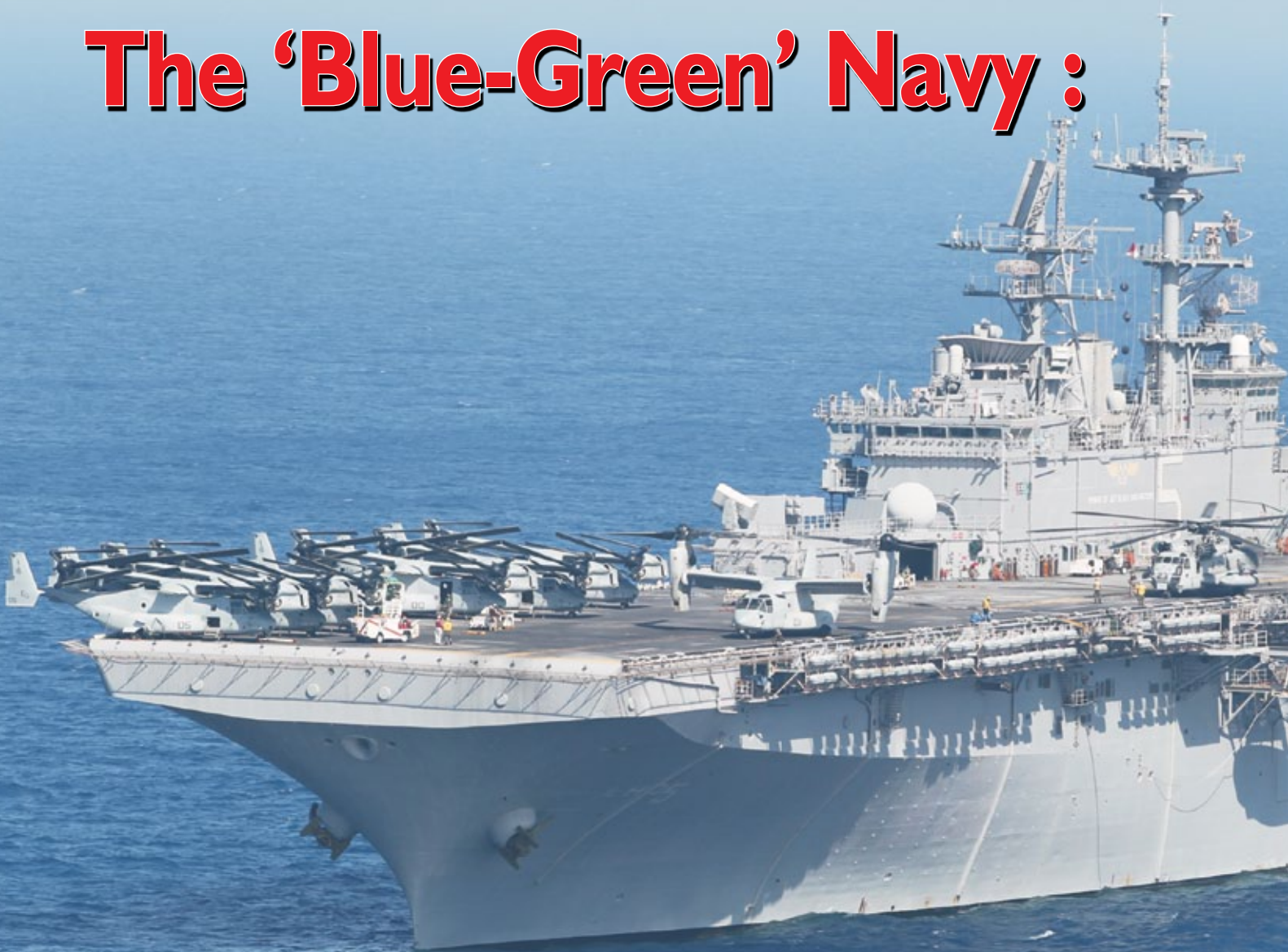
The USS Bataan is a Wasp class Landing Helicopter Dock (LHD) amphibious assault ship. The design is based on the Tarawa class, with modifications to operate more advanced aircraft and landing craft. The Wasp class is capable of transporting almost the full strength of a United States Marine Corps Marine Expeditionary Unit (MEU). In total eight Wasp-class ships have been built since 1989.
