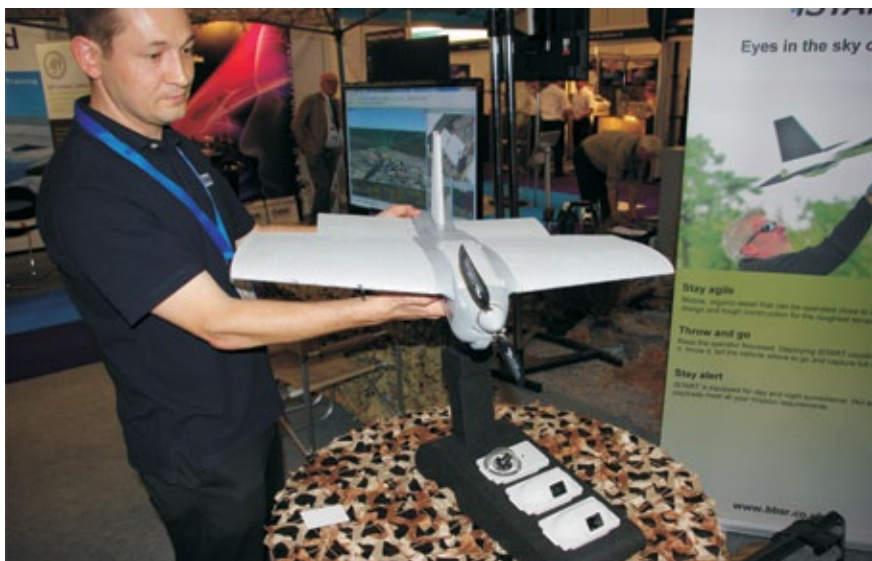
The Bluebear iSTART was one of the smaller UAVs at the show and can fit, with its laptop-size control console in the boot of a car. It can also be fitted with different payload packages. Once launched by hand, the mini-UAV operates autonomously and distributes a live image back to the operator.
