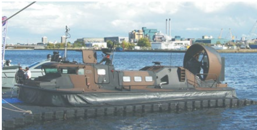
The show included warships and hovercraft, such as this Griffin hovercraft, which has been ordered by the UK's Royal Marines for high speed assault duties and can be carried aboard assault landing platform / helicopter ships.
