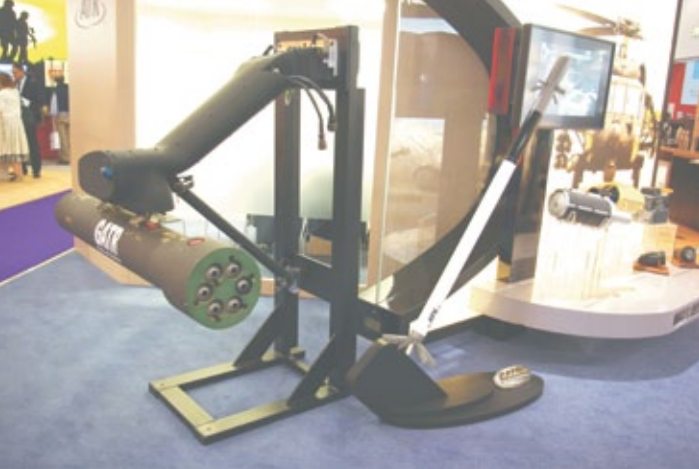
Another similar precision weapon, based on a rocket is the ATK GATR, seen in its launch pod (left) and on its own (right).
