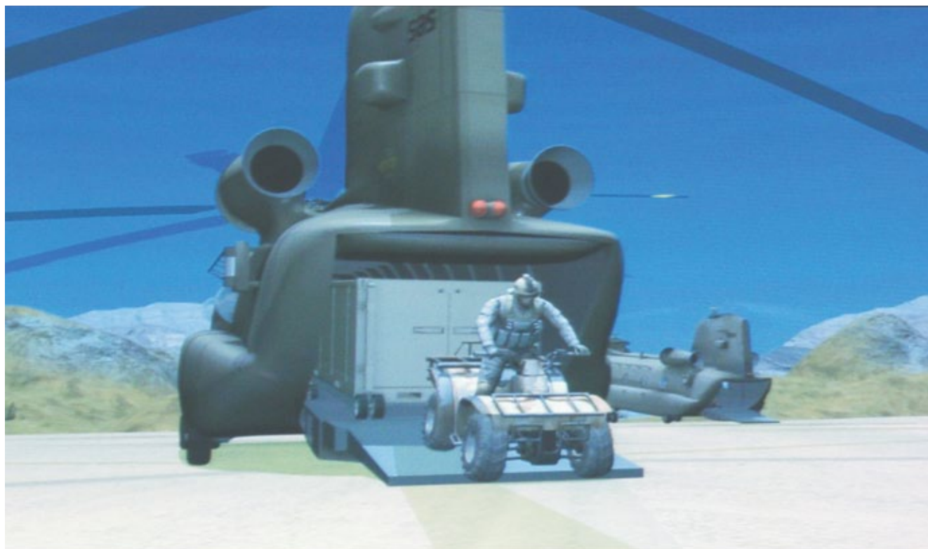
Weatherhaven has developed an innovative expanding container system, TRECC, which can be carried inside a CH-47 Chinook and which can open up to provide a field medical centre or combat HQ. This allows safer and faster air mobility by helicopters compared to conventional underslung loading of containerised shelters and other equipment.
