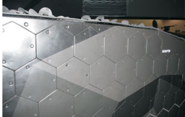
These innovative tiles, part of BAE Systems Adaptive electronic camouflage project, seen here fitted to an armoured personnel carrier can also be produced for other vehicles, and could later be adapted for use on warships and helicopters. Small video cameras monitor the background IR signatures and the tiles can be programmed to reproduce a similar signature, creating an effective masking cloak that makes the vehicle invisible to other IR sensors on the battlefield.
