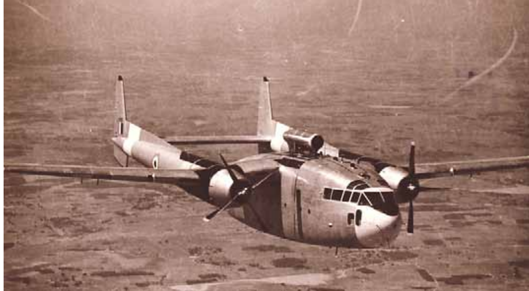
Fairchild C-119G Packet with dorsal mounted jet engine for augmenting power, was obsolescent by the mid-70s.
