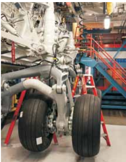
Main wheels of 'India 1' landing gear : the C-17's landing gear system consists of a single nose strut with two wheels and two twin-strut tandem gear assemblies, one per side with three wheels per strut.
