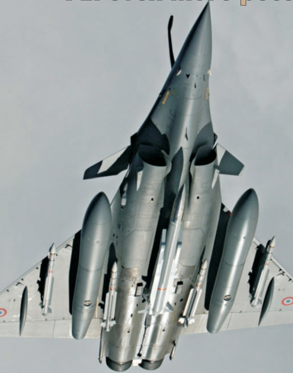
Extremely rare view of a French Air Force Rafale B with a single MBDA 3 kiloton ASMPA thermonuclear missile in the central position, plus 4 MBDA Mica air-to-air missiles. The aircraft is in full nuclear strike configuration with a pair of 2,200 litre drop tanks. Pictures with nuclear weapons are hard to come by. (Official Armée de l'Air photo - SIRPA-Air)
