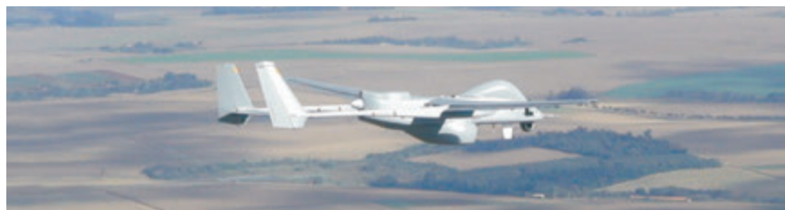
IAI's Heron with satellite communication, electro optic, maritime radar, COMINT and ELINT payloads
