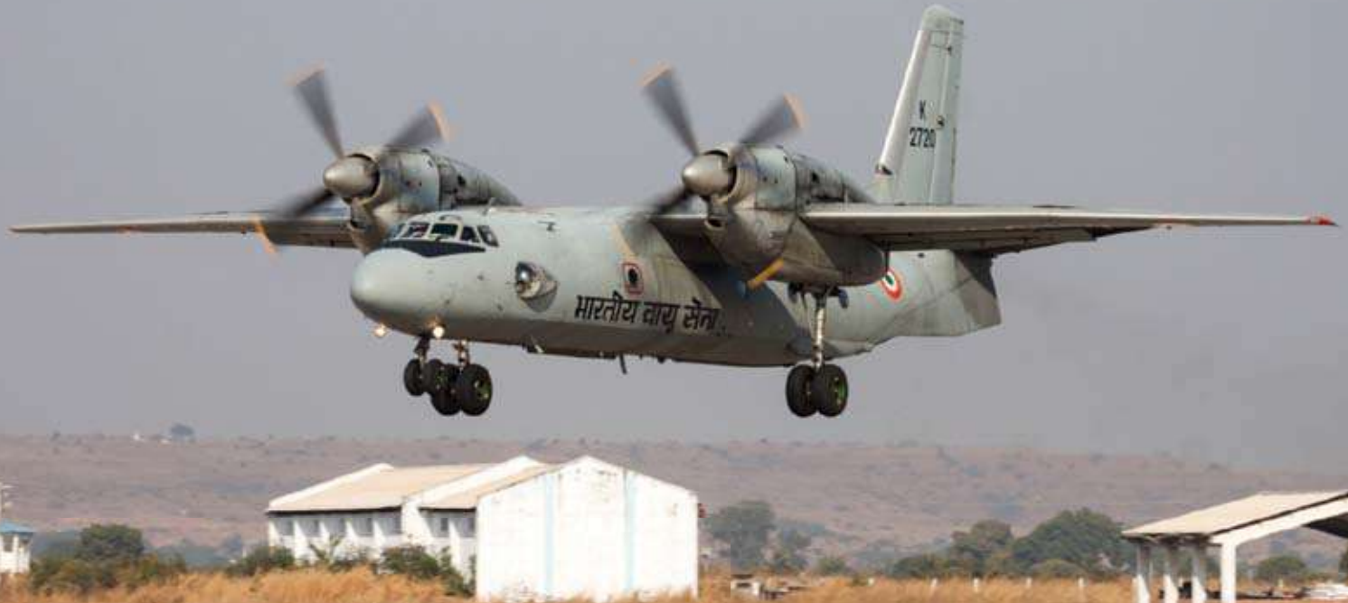
Powered by two massive Ivchenko AI-20M turboprops of 4,195 shp each, an An-32 comes in to land at Gwalior with its long concrete runways. The An-32 is essentially an An-26 with more powerful engines and larger propellers for augmenting performance from 'hot and high' airfields in the mountainous terrain of north and north-east India (photo: Angad Singh)
