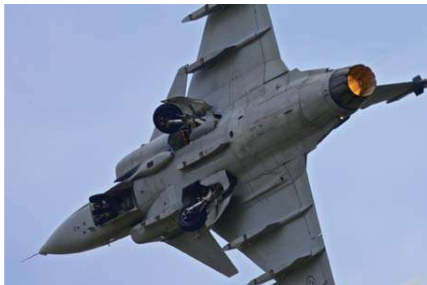
The Gripen C is powered by a single Volvo RM12 (GE F404) producing 8,200 kg thrust with afterburner (photo: Peter Gronemann)
