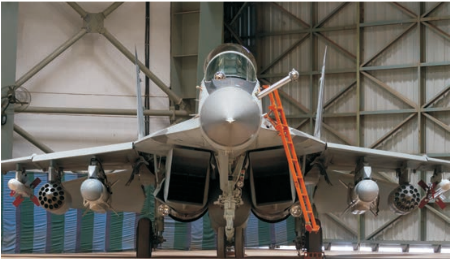
Indian Navy MiG-29K with its weaponry seen on six underwing hardpoints (photo : Angad Singh)
