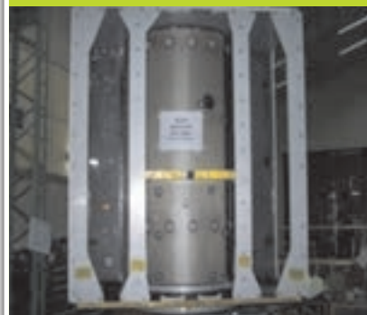
The Mars Orbiter Mission Satellite Structure (Bare structure supplied by HAL)
