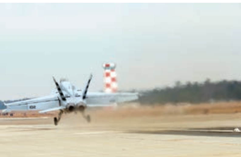
A US Navy F/A-18E Super Hornet launches during a land-based EMALS test (US Navy photo)
