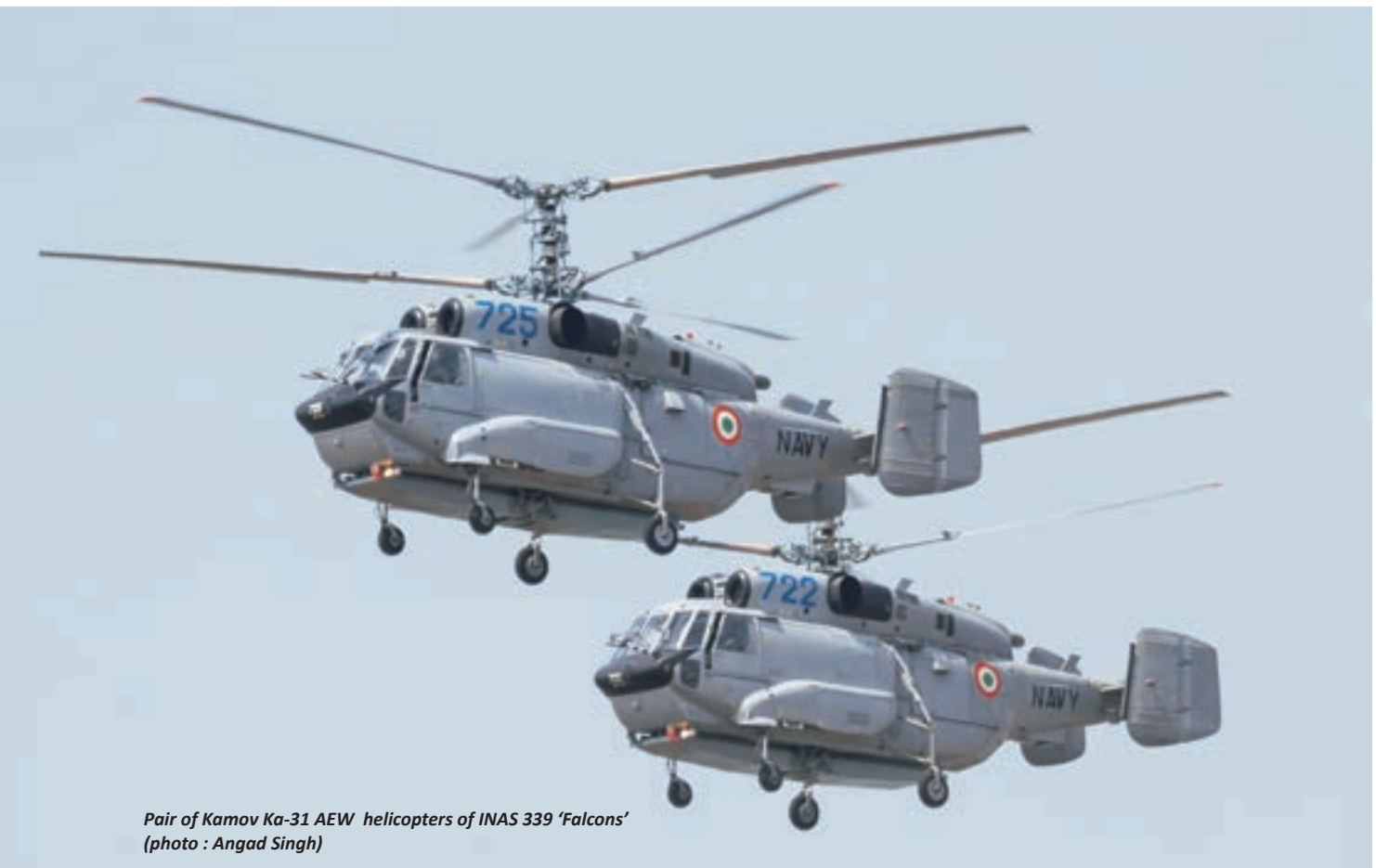
The Kamov Ka-31AEW helicopter is operated from warships by the Indian Navy for airborne early warning
