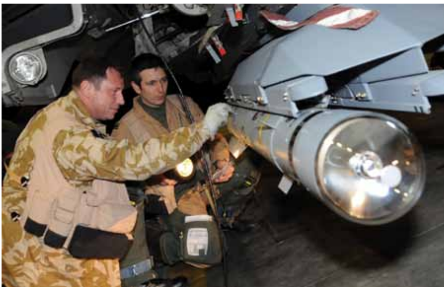
A Dual-Mode Brimstone missile being loaded on a triple ejector rack (TER) under a Panavia Tornado (MBDA photo)
