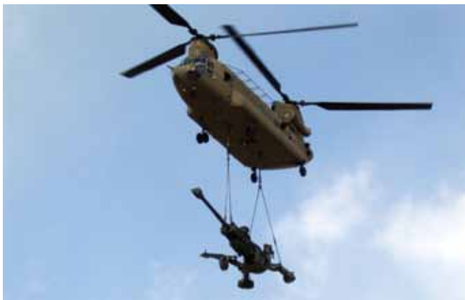
The Boeing Chinook, powered by twin Lycoming T-55 turboshafts, boasts an impressive airlift capability in the high mountains, as proved in Afghanistan.
