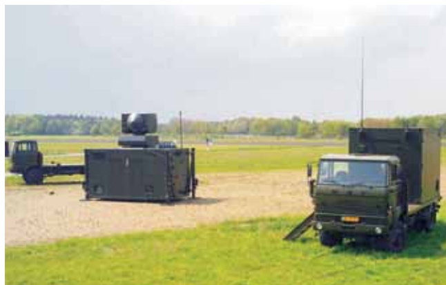
A combined surveillance and track radar is the best way to ensure quick and unambiguous hand-over from surveillance to track radar. The Combined Antenna System shortens the deployment time and allows both sensors to see in all directions simultaneously, without blanking, contrary to non-combined sensor configurations (photo: Thales)
