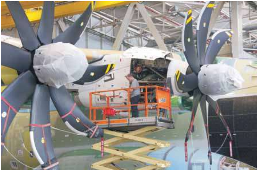
A technician checks the engines in the assembly line. The A400M is powered by four counter-rotating TP400 turboprop powerplants.
