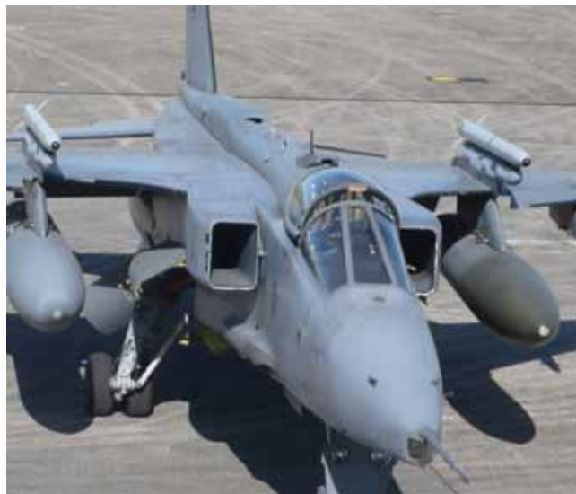
Inert ASRAAMs mounted on an ex-RAF Jaguar during trials (MBDA photo)
