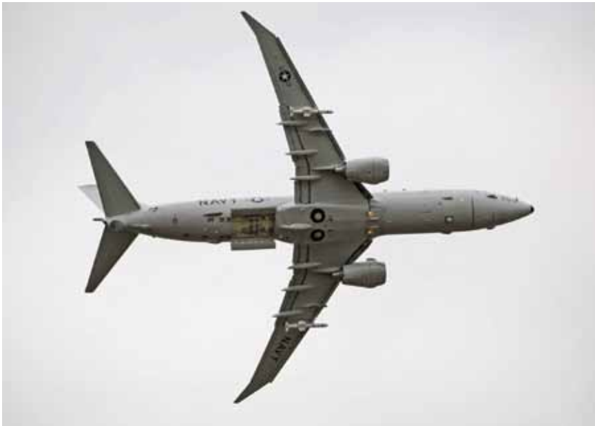
US Navy Boeing P-8A from Air Test and Evaluation Squadron ONE (VX-1) conducted displays armed with inert AGM-84 Harpoon ASHMs mounted underwing
