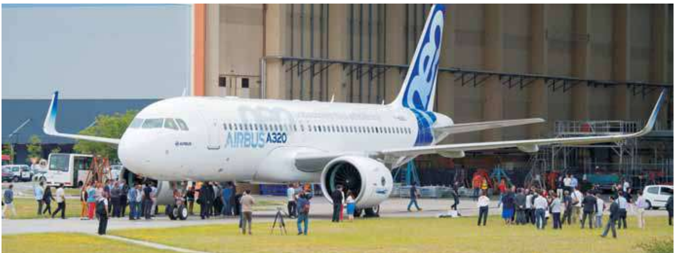
The assembly of Airbus' first A320neo has been completed following painting of the aircraft and mounting of Pratt & Whitney PW1100G-JM engines. MSN6101, which will be the first A320neo to fly, will shortly start its ground tests to prepare for first flight.
