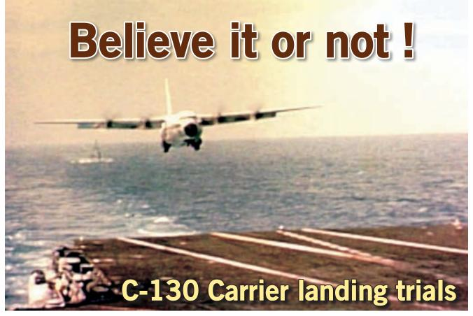
Image taken from video of the KC-130F coming in for a landing on the USS 'Forrestal' in the fall of 1963. The US Navy aircrew in this KC-130 tanker would make twenty-nine touch-and-go landings and twenty-one full stop landings at increasingly heavier weights on three flights to the carrier
