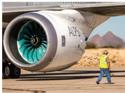
a variable pitch fan system, is based on technology that could be ready for service from 2025 and will offer at least 25 per cent less fuel and  $CO_2$  emissions against the same baseline. CTi technology delivers lighter fan blades while retaining aerodynamic performance.
