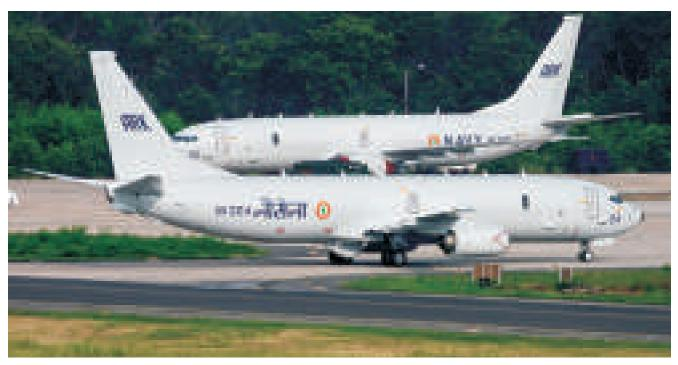
Radome for the aft radar and the slender MAD boom can be seen in this image as IN324 taxis back to the apron
