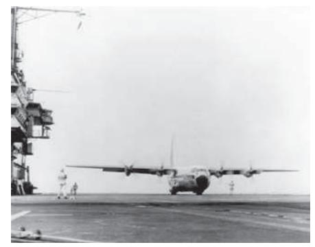
On 8 November 1963, after making the three warm-up touch-and-go landings, Lt. Jim Flatley was cleared for the first full stop landing. The aircraft stopped in 275 feet, actually short of where the number four arresting cable would have been lying. Here, the aircraft is readied for takeoff on the deck of the 'Forrestal' after a full stop landing
