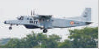
Dornier 228 of INAS 311 taking off, with ESM antennae visible on the wingtips, search radar in a dark underbelly radome, and AMOSP just ahead of the mainwheels
