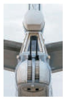
The tail turret is seen to good effect in this image, along with the white radome of the aft fire control radar
