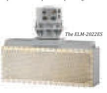
and processing algorithms of the ELM-2022 family, while using the unique capabilities of Active Electronically Scanned Array (AESA) technology. The radar system combines mechanical scan in the horizontal plane with fine beam shifting, and full electronic scan in the vertical plane, providing improved detection, particularly at high sea states.
