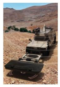
consists of an ADS (Above-surface Detection System), and MIDS (underground Mine and IED Detection System). The ADS includes a groundbreaking side-looking SAR radar, high-resolution optical detection system and an infrared multispectral investigation system. MIDS comprises a Ground Penetrating Radar (GPR) and a magnetic detector.
