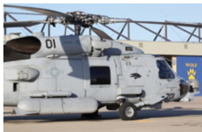
MH-60R with external fuel tank on hardpoint
