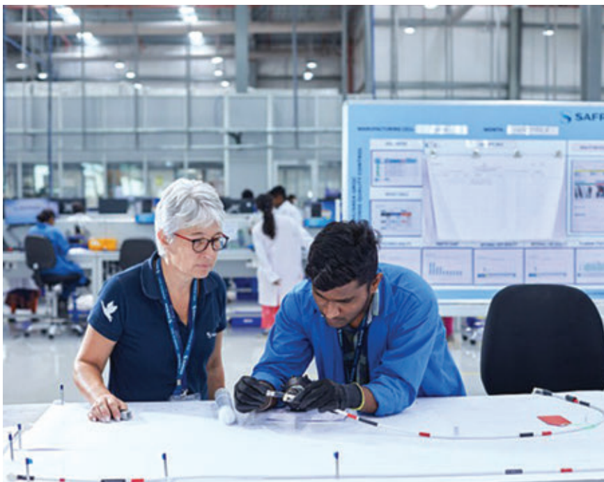
Harness Inspection on the Rafale production line at Safran facility in Hyderabad, India. (photo: Christophe Viseux / CAPA Pictures / Safran)
