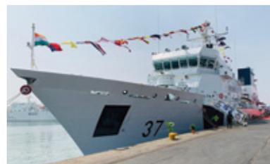
at Kattupalli, Chennai and is fitted with state-of-the-art navigation and communication equipment, sensors and machinery. The ship will be equipped with 30mm and 12.7mm guns with Fire Control System for enhancing its fighting efficiency. The ship draws 2100 tons (GRT) and is propelled by twin MTU 8000 series engines of 9100 KW each, capable of achieving 26 knots of top speed and endurance of 5000 nm at economical speed.
