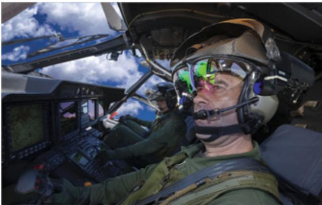
NHIndustries has chosen the new-generation TopOwl Digital Display helmet from Thales for the Special Forces variant of the NH90 helicopter. This variant has been developed at the request of the French defence procurement agency (DGA) to meet the requirements of France's Special Forces, and is also available to partner countries and other NH90 customers.
