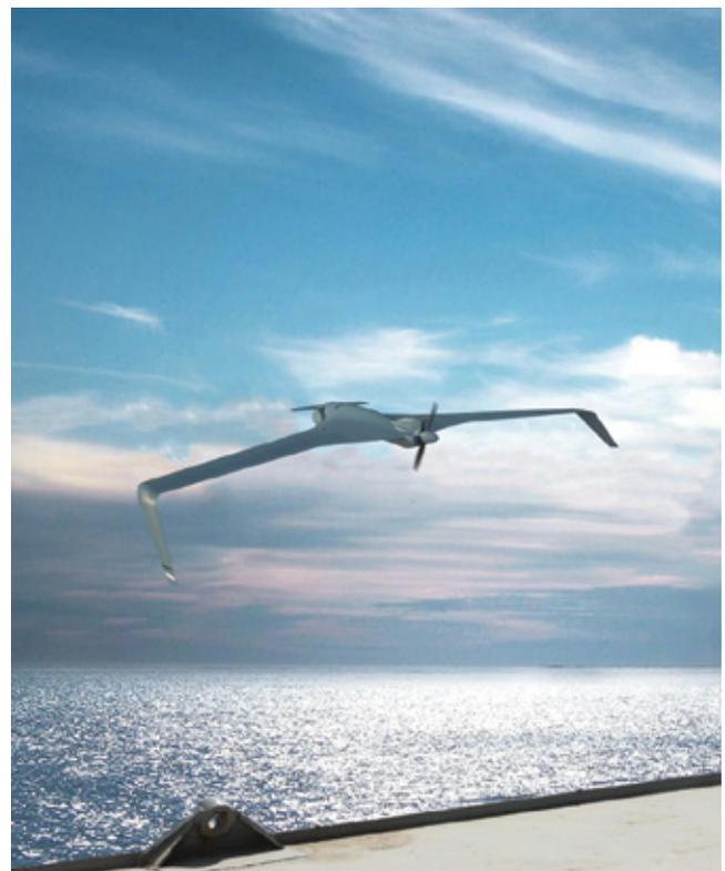
Aeronautics Group has introduced its Orbiter 4 small tactical AUAS, capable of performing long-range, long-endurance maritime patrol missions. The Orbiter 4's high-performance EO/IR and MPR payloads are ideal for maritime monitoring, gas and oil rigs protection, illegal activity tracking, and search & rescue. It has already been fully integrated into the operational environment of navy vessels, and meets the requirements of navy operations.
