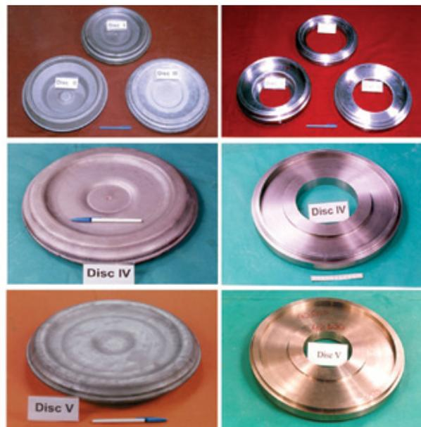
produced and successfully supplied to HAL for fitment in to Adour Engine that powers the Jaguar/Hawk aircraft.
