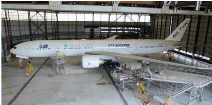
Development Programme for the 777-300ERSF. This is a key milestone for "the Big Twin," the GECAS-IAI Co investment for the passenger-to-freighter conversion program of the GE-90 powered 777-300ER, as it now moves beyond planning into the phase of physically modifying the aircraft
