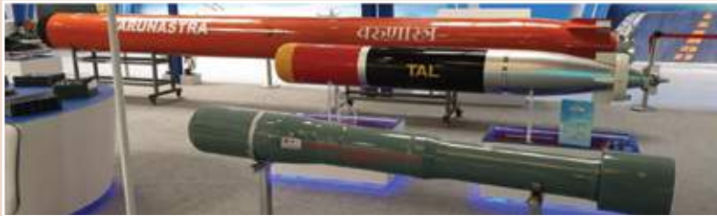
Top Down: BDL produced Varunastra ship-launched heavy weight electrically-propelled anti-submarine torpedo; light weight anti-submarine torpedo (TAL); extended range anti-submarine rocket (ER-ASR)
