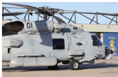
MH-60R with external fuel tank on hardpoint
