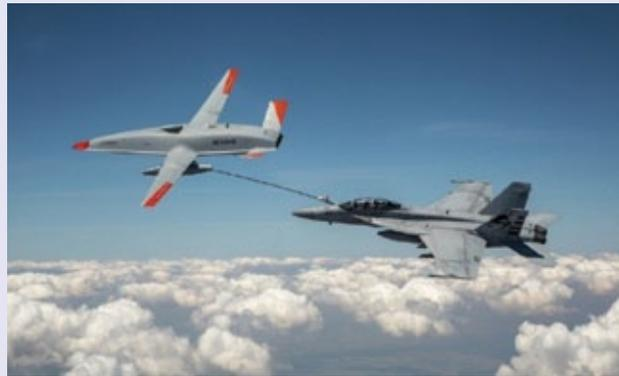
safely completed, the MQ-25 drogue was extended, and the F/A-18 pilot moved in to “plug” with the unmanned aircraft and receive the scheduled fuel offload.
