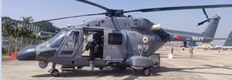
has a battery backup of four hours. The equipment can be installed in two-three hours to convert the aircraft into an air ambulance. This is the first of eight MICU sets to be delivered by HAL to Indian Navy.
