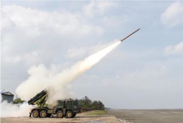
Chandipur off the coast of Odisha. Twenty-five Enhanced Pinaka Rockets were launched in quick succession against targets at different ranges. The enhanced range version of Pinaka Rocket System can destroy targets at distances up to 45 kms. All the flight articles were tracked by range instruments including Telemetry, Radar and Electro Optical Tracking System deployed by ITR & Proof and Experimental Establishment (PXE).
