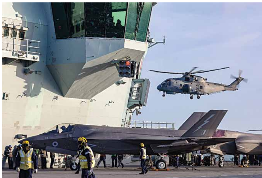
A Merlin helicopter fitted with Crowsnest early warning and surveillance system taking off with radar in the retracted position (Crown Copyright RN21 photo)
