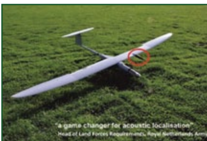
Figure 4: Acoustic Localisation Sensor (Image courtesy Microflown AVISA)
