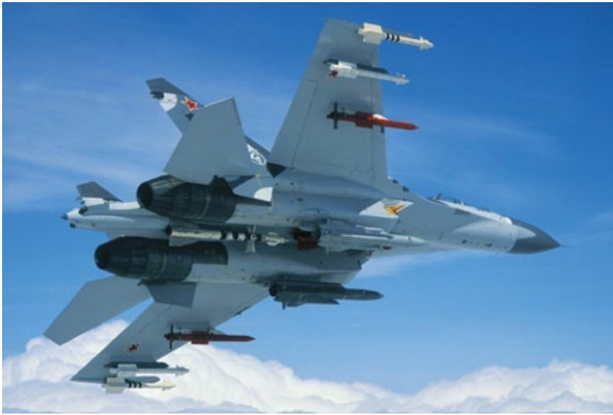
RuAF Su-27 equipped with Kh-31, R-27, R-73 and R-77 missiles (Photo: NPO Saturn)
