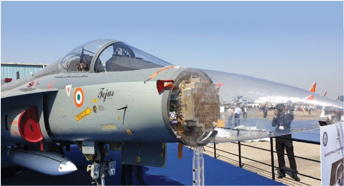
Mockup of the Uttam Active Electronically Scanned Array Radar (AESAR) on the Tejas
