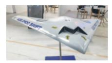
The Unmanned Aerial Vehicle is designed and developed by Aeronautical Development Establishment (ADE), Bengaluru, a premier research laboratory of DRDO. It is powered by a small turbofan engine. The airframe, undercarriage and entire flight control and avionics systems
