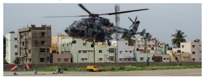
The first flight of Advanced Light Helicopter (Wheeled Version) with segmented MRBs (Main Rotor Blades) and MRH (Main Rotor Head) in pre-cone configuration was carried out in Bengaluru on 30 June 2022. The flight was carried out by Wg. Cdr. Unni Pillai, ED (CTP-RW).
