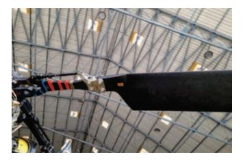
available in Indian Navy ships. Segmented blade feature reduces the folded length and width of ALH making it compatible with the hangar space available on most of the Indian Navy ships. Further, the time required for folding or unfolding operations is reduced.
