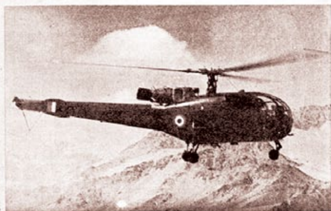
GETTING TO THE TOP. The IAF helicopter wing has been doing tremendously good work across the Himalayan range. The French-built Alouette is usually reserved for evacuation of casualties. It can climb to 19,000 ft and has a speed of 100 m.p.h. The IAF also has the smaller Russian Mi-4s and the older S-55 and S-62 helicopters. Our total 'copter strength is about 130. And India holds the world record (22,500 ft)—in an Alouette piloted by K. K. Saini.
