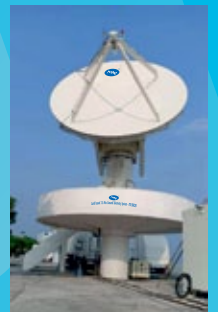
Land based 7.3 mtr Ground Telemetry system
