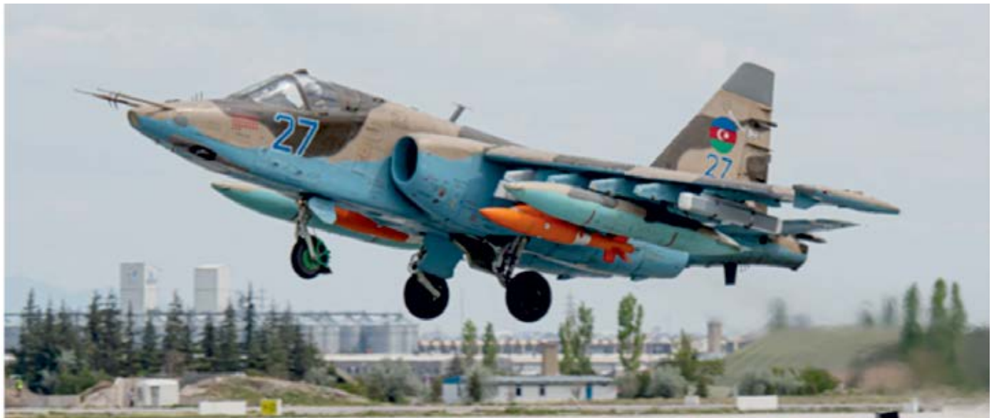
A Su-25 takes off with a pair of 1000 lb bombs fitted with Wing Assistance Guidance Kits produced by TUBITAK SAGE.
