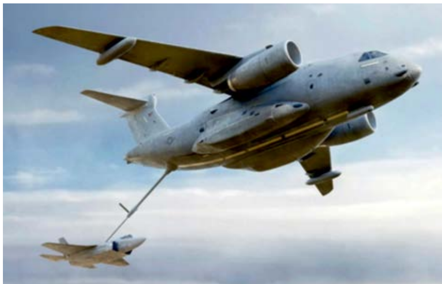
A drawing of the proposed boom configuration. This will expand the air to air refueling possibilities for the KC-390 and open up for potential new customers (Photo: Embraer)
