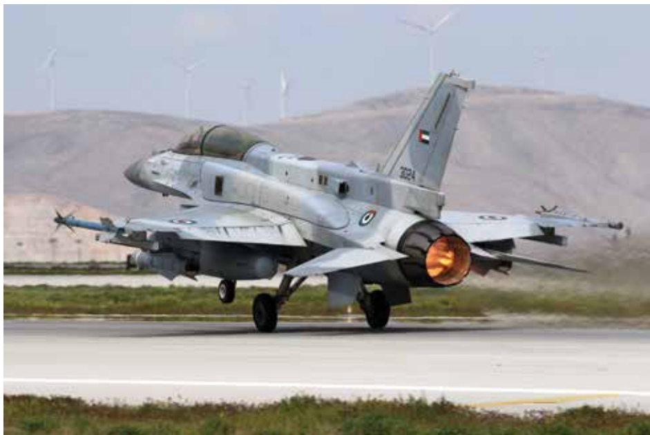
UAE Air Force block-52 F-16F armed with an AGM-65 “Maverick” missile
