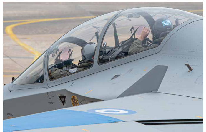
A close look in the office. The current HUD will be replaced with a low profile version which will be integrated with the new single display.
