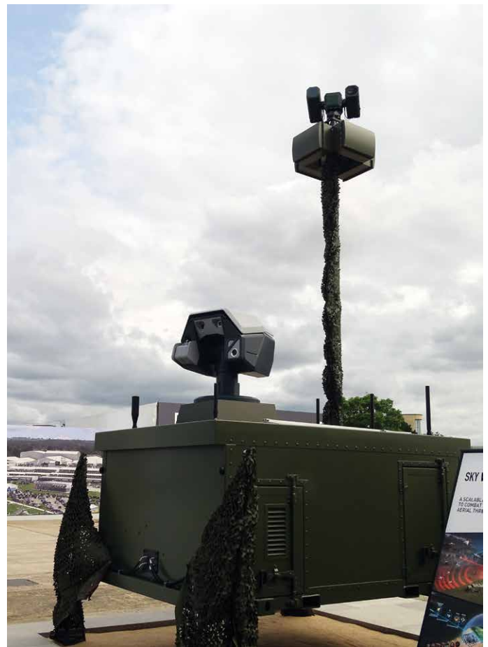
MBDA Sky Warden anti-drone mobile unit with laser effector and telescopic mast with 360 D radar, EO and IR sensors on the mast.
