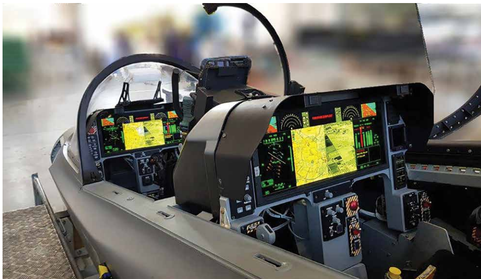
An early rendering of how the cockpit of the M-346 Block 20 could look like with the proposed large single display-Leonardo.
