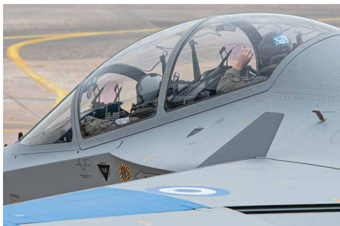
A close look in the office. The current HUD will be replaced with a low profile version which will be integrated with the new single display.
