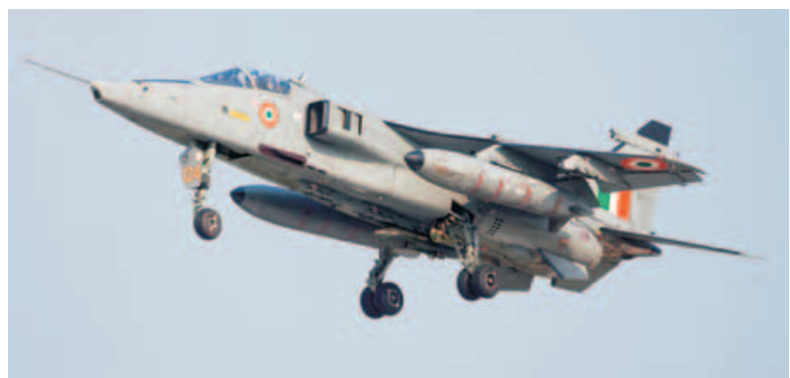
DARIN II Jaguar (note RWR and reprofiled nose) seen on approach for landing (photo: Angad Singh)
