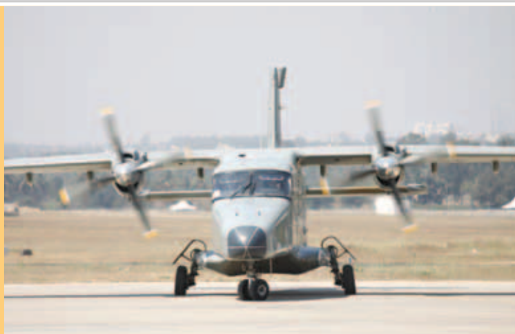
The HAL Dornier 228, built at Kanpur, can carry 19 passengers and has excellent short take off and landing performance which makes it ideal for flying to hitherto unconnected airfields throughout India and particularly in mountainous terrain and offshore islands
