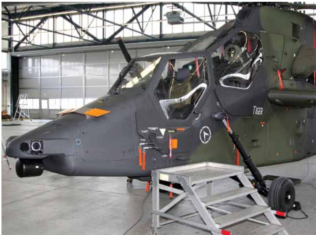
Tiger helicopter being tested with additional cockpit protective plating
