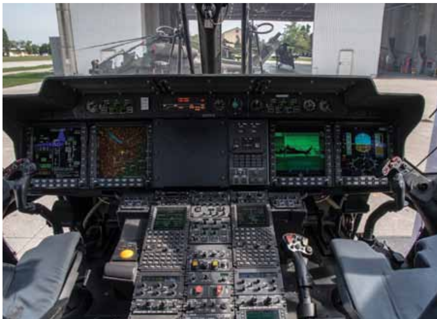
A cockpit view of the UH-90A clearly showing the multi-functional colour screens
