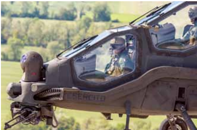
The gunner uses the helmet mount sight for the M197 three-barrel Gatling-type cannon
