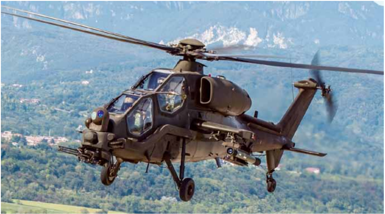
The AH-129D was introduced in 2014 and includes a new targeting system incorporated in the nose turret
