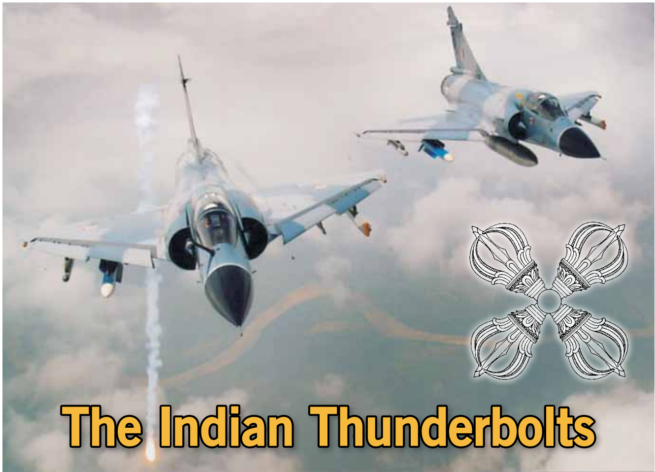
Pair of IAF Mirage 2000s with Super 530D BVR and Magic II missiles and firing infrared flares (inset ; depiction of the Vajra weapon)
