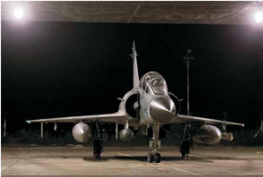
Mirage 2000TH with Litening pod on starboard fuselage pylon and Remora ECM pod on port wing (photo: Angad Singh)
