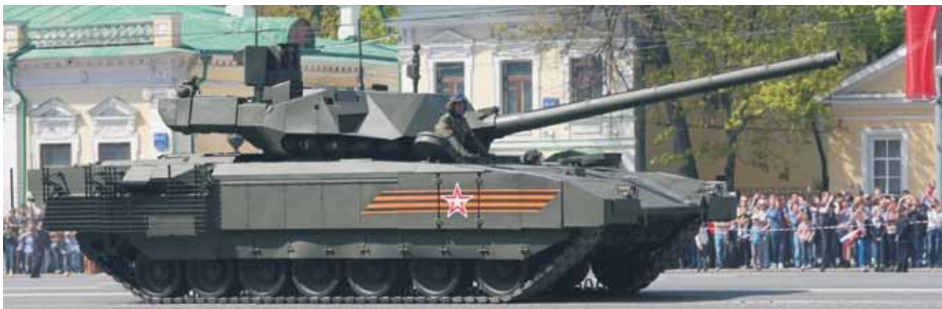
T-14 Armata MBT, displaying radical new profile, including unmanned turret, new track configuration, and commander seated in the hull (photo: Sokolrus)
