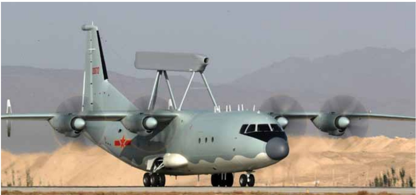
The KJ-200 AEW&C aircraft incorporates an AESA radar system, mounted on a top fuselage beam. The aircraft is based on the Y-8 transport aircraft, itself based on the An-12 but with Pratt & Whitney Canada PW150B turboprops
