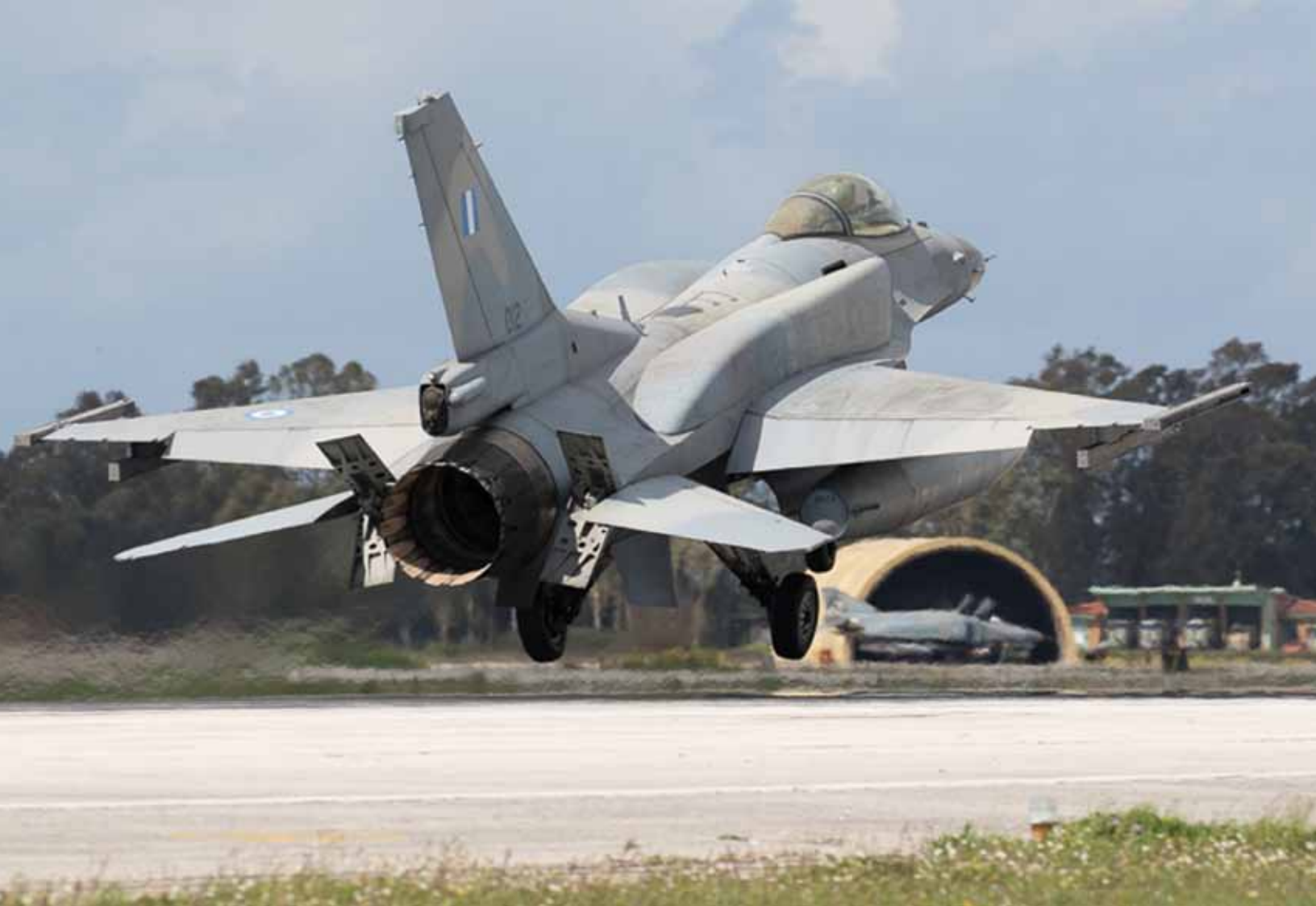
Using conformal tanks to extend mission time, this Greek F-16C returns back to Andravida
