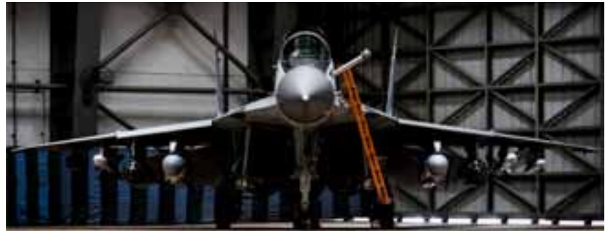
Indian Navy MiG-29K showing armament load, including two Kh-35 ASHMs on the inboard pylons (photo: Angad Singh)
