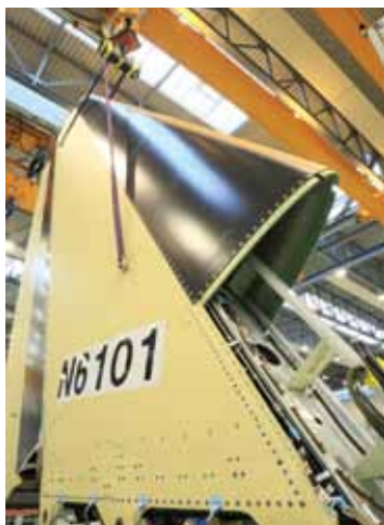
NEO vertical tailplane produced at Stade
