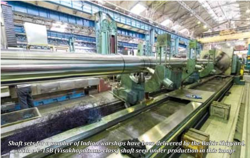
Shaft sets for a number of Indian warships have been delivered by the Baltic Shipyard, with a P-15B (Visakhapatnam-class) shaft seen under production in this image
