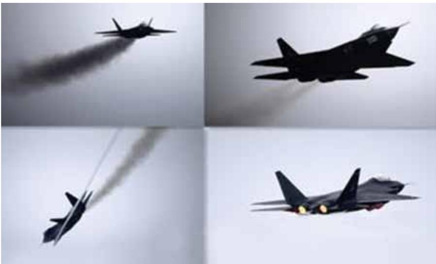
*Black smoke from the Russian RD-93 engine is very visible during various maneuvers from the J-31. China is looking out for a potential replacement engine for the J-31*
