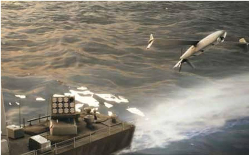
electro-optically guided munition has a loitering time of 90 minutes, during which its operator can collect visual intelligence of surrounding area areas – especially in congested waters and shore targets at a range of up to 40 km.
