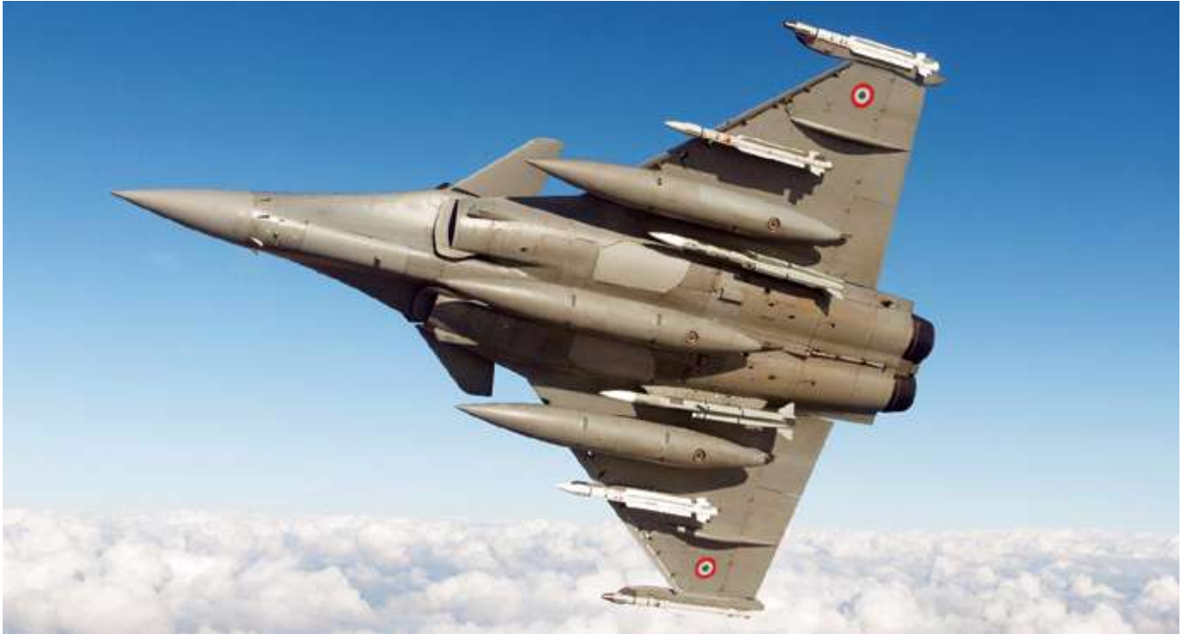
French Air Force Rafale (in this photo) but soon to be in Indian skies with the IAF as an operator of the type, is seen here with two MBDA Meteor's and four MICA AAMs. (photo: Dassault)
