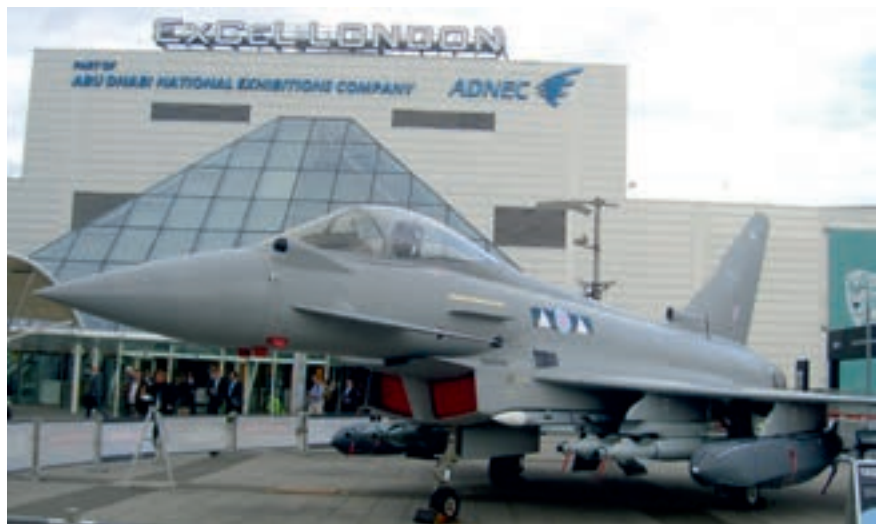
An operational RAF Typhoon FGR4 on static display fitted with cruise missiles, LGBs, Brimstone PGMs and Meteor BVRAAMS
