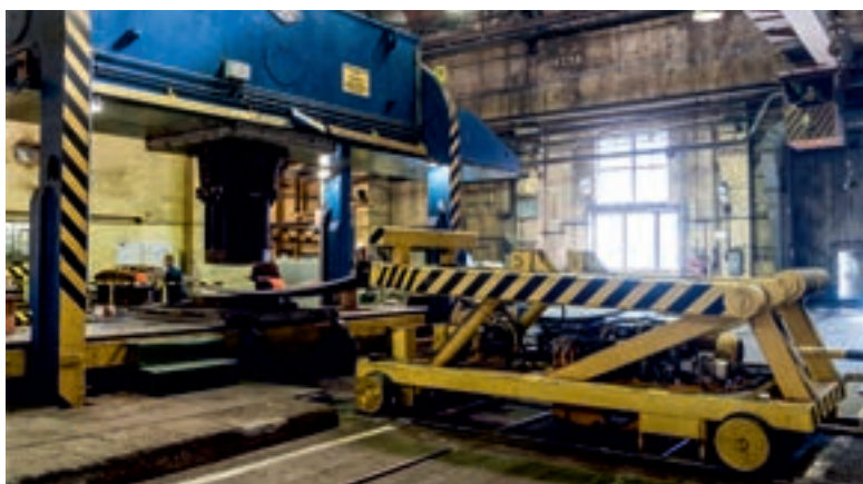
An incredibly powerful hydraulic hammer gives just the right curvature to dozens of steel plates so that they can be welded into watertight submarine pressure hulls
