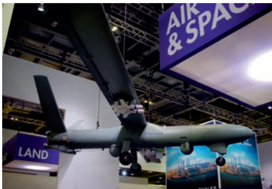
Thales Watchkeeper model at the show, fitted with FFLMM glide bombs
