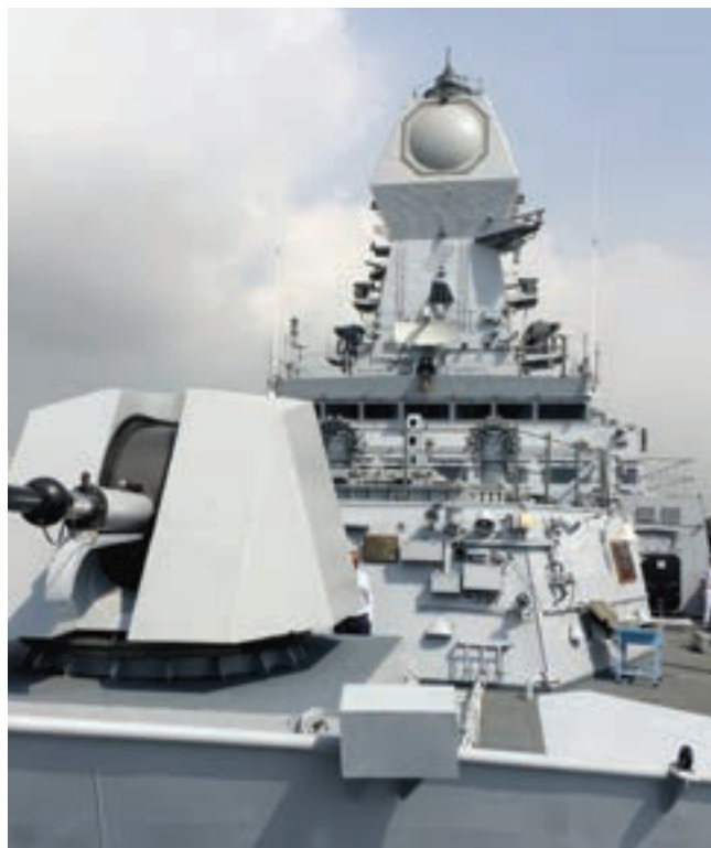
INS Kochi's 76mm Oto Melara Super Rapid Gun Mount in the foreground with the large IAI Elta EL/M-2248 MF-STAR phased array radar visible on top of the mast
