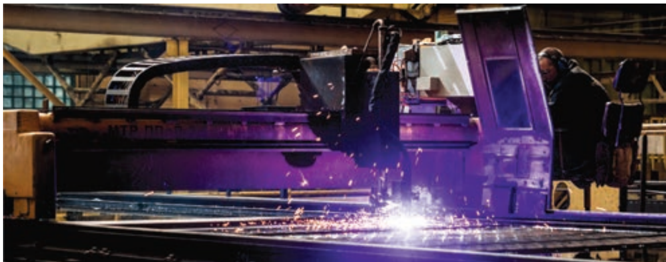
Admiralty Shipyards uses different types of cutting methods for different applications — from plasma cutters as seen above...
