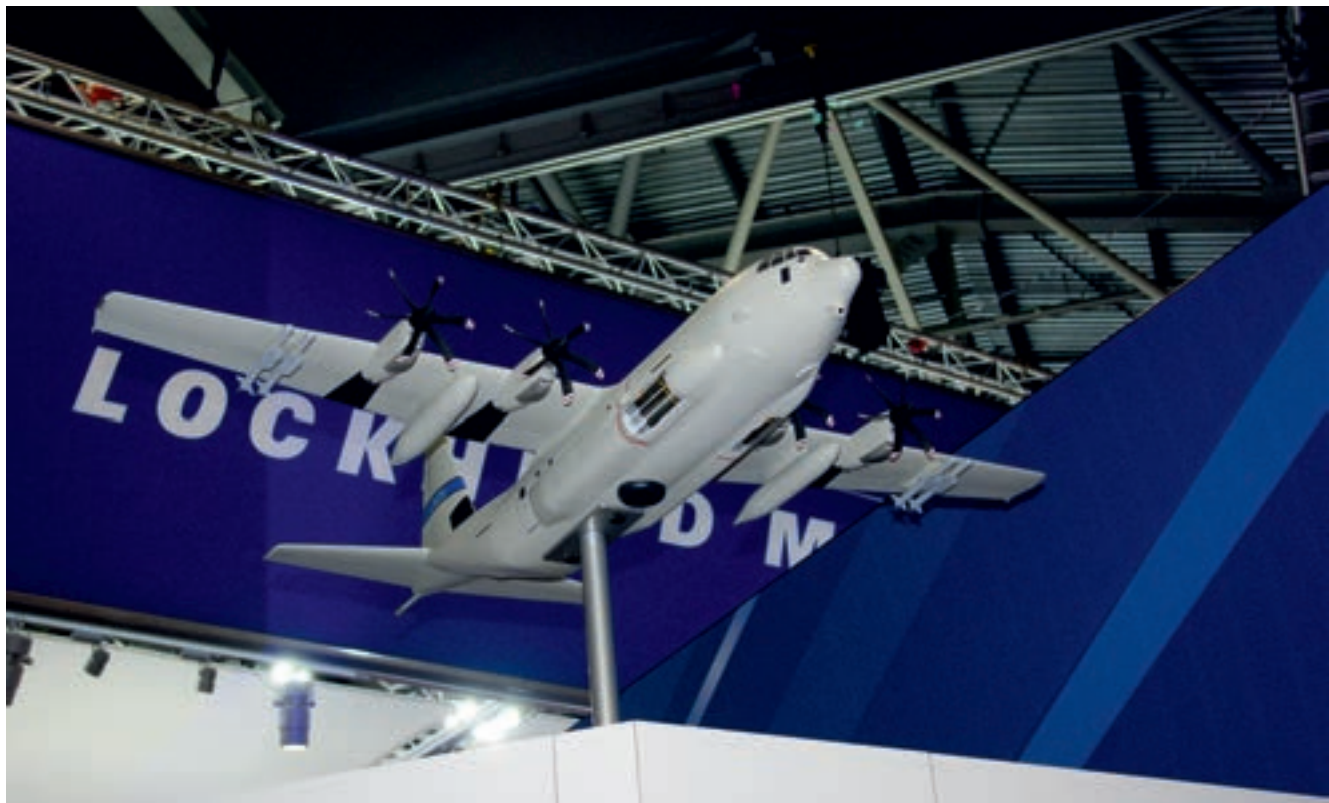
Lockheed Martin SC-130J model showing search radar and electro-optical turret, ASHMs, MAD boom, and weapons bays housed in enlarged sponsons
