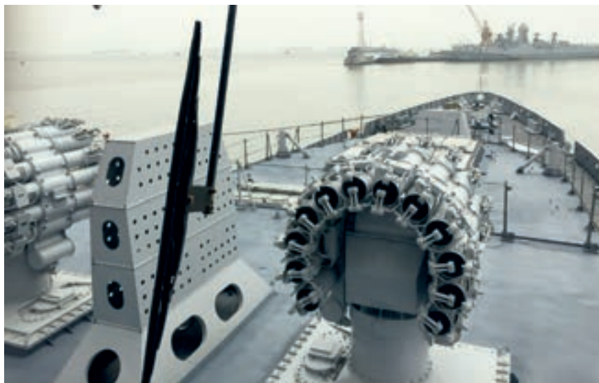
INS Kochi's RBU-6000 anti-submarine rocket launcher, LR-SAM and Brahmos vertical launch cells, and 76mm main gun visible from the bridge, while its sister ship is seen moored in the distance
