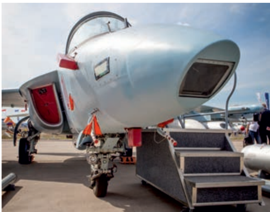
Aperture of the laser rangefinder on the nose of a modified Yak-130 at MAKS 2015
