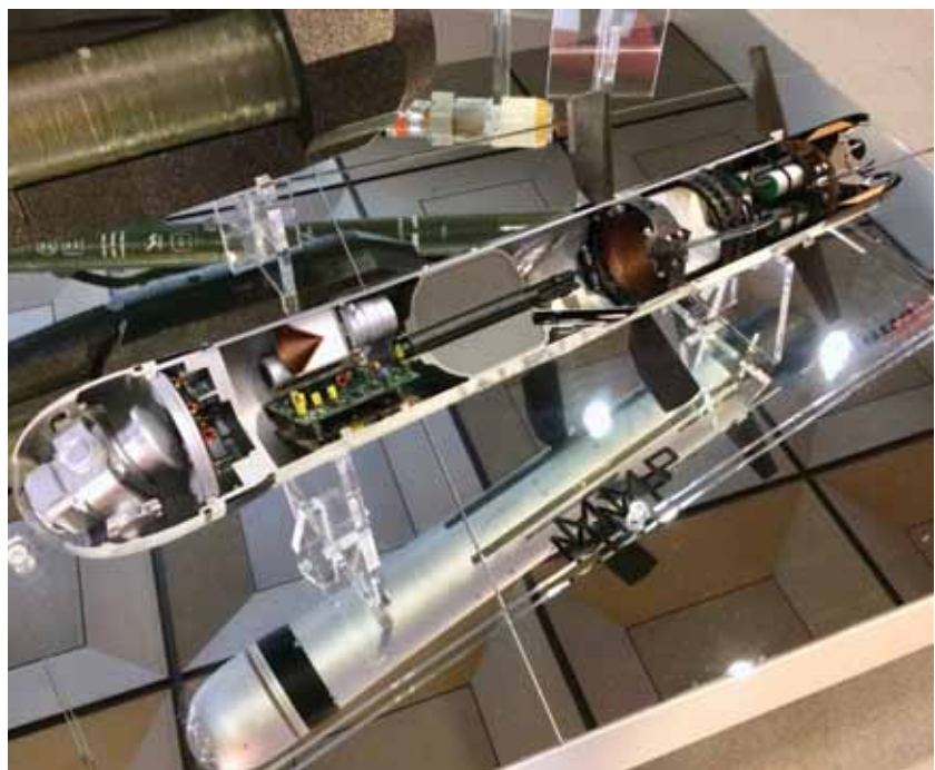
Cutaway model of the MMP at MBDA's Selles-Saint-Denis production site, showing tandem warheads, mid-body motor, as well as seeker and guidance hardware (photo: Angad Singh)
