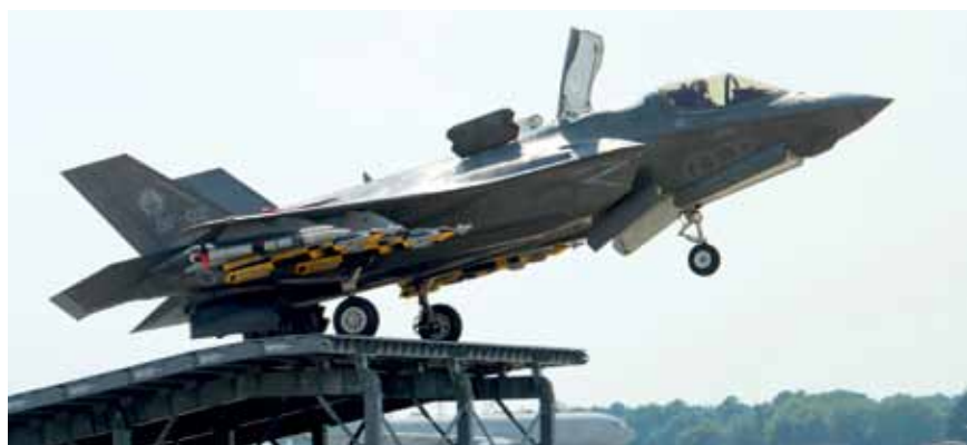
An F-35B development aircraft carries out ski-jump testing with external stores, as required by the UK customer (photo: Arnel Parker)
