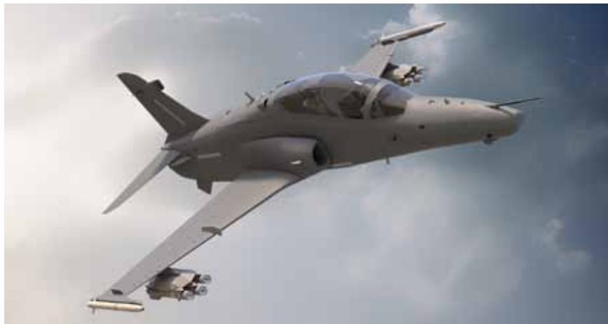
A render of a Hawk Mk.132 armed with ASRAAM on the wingtips and two Brimstone triple racks
