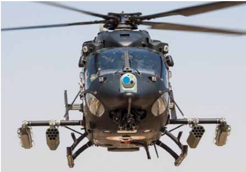
Mistral twin-missile launchers seen on the outboard weapon stations of this Indian Army Rudra helicopter (photo: Angad Singh)
