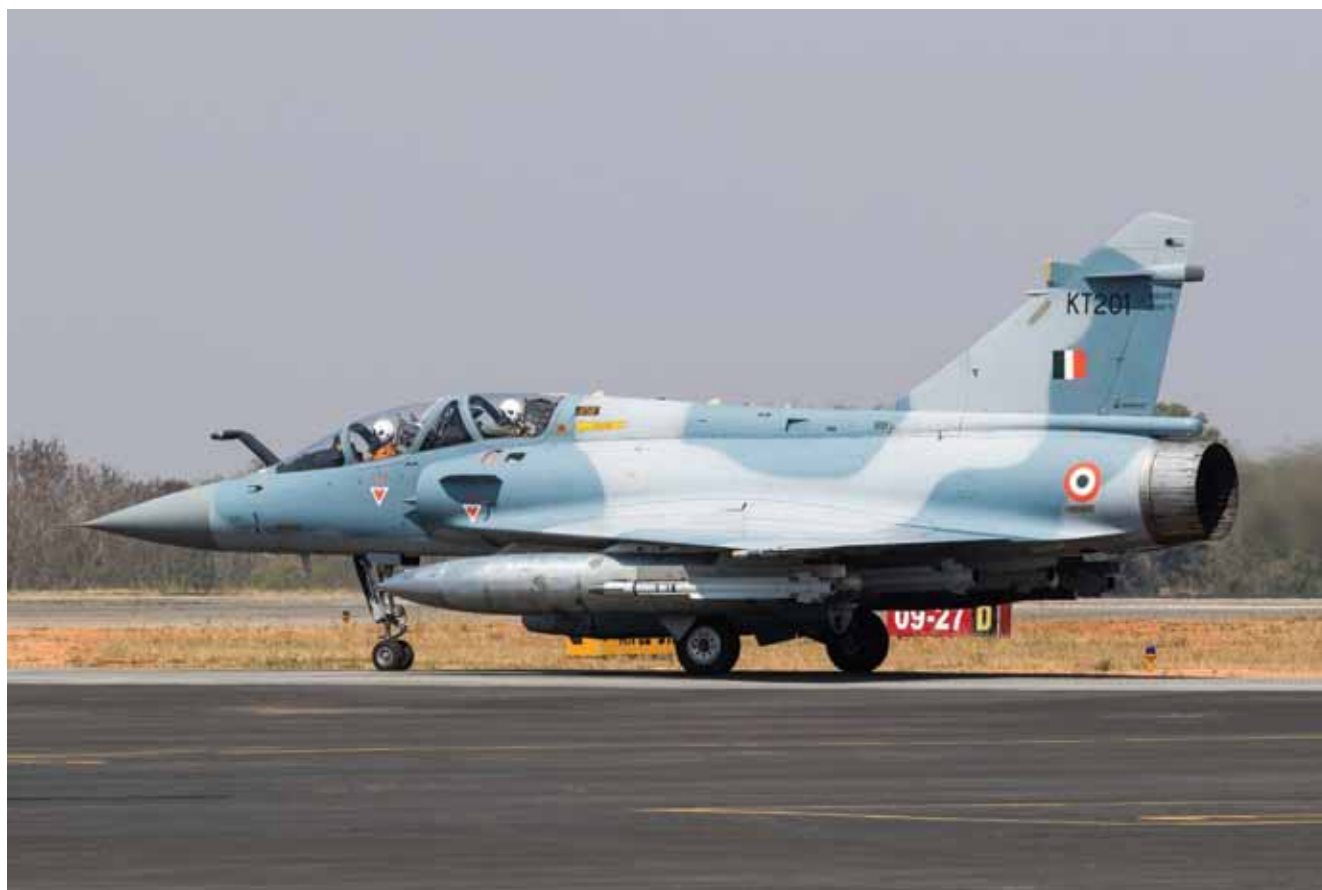
Upgraded IAF Mirage seen taxiing with five MICA missiles, three on wingroot stations, two on outboard wing stations (photo: Angad Singh)
