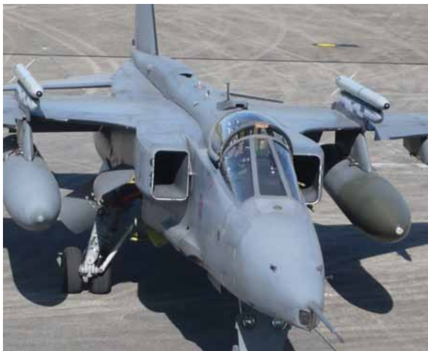
Inert ASRAAMs mounted on an ex-RAF Jaguar during trials (photo: MBDA)
