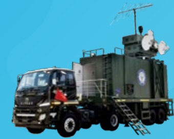
Radiation Mode Test & Evaluation Facility for Radar EW Systems
